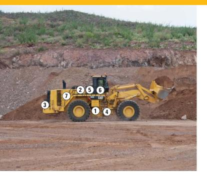
The 992K is organized into individual service centers. Combined with the diagnostics available through VIMS, Product Link and Electronic Technician, servicing the 992K can be simple and efficient.
