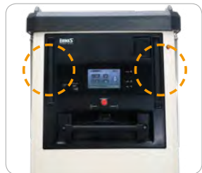
Emergency stop button and front collision sensor In case of an emergency, the operator can stop the cart with the emergency stop button. In addition, the front collision sensor automatically stops the cart in case of a collision.
