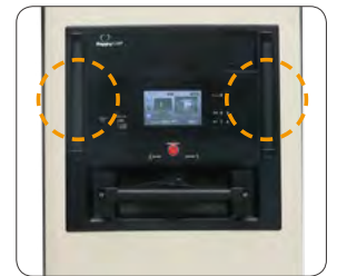
Emergency stop button and front touch sensor In case of an emergency, the operator can stop the cart with the emergency stop button. Touching the front touch sensor lowers the speed when the user requires.
