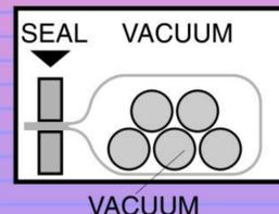
When the desired vacuum is reached the seal bar closes to seal the bag.
