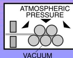
Atmospheric pressure is restored to the chamber and causes the bag to cling to its contents.
