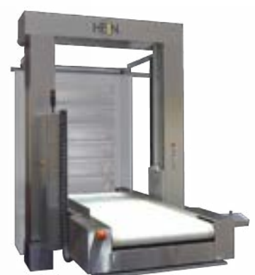
Example of a customised system: 4 HEIN ELECTRO deck oven with six decks each and the fully automatic HEIN SPIDER loading and unloading system.
