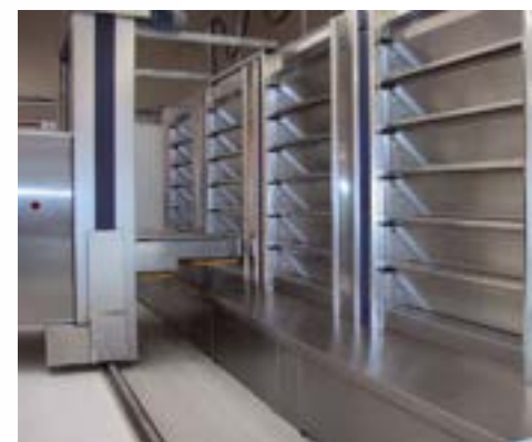
Example of a customised system: 4 HEIN ELECTRO deck oven with six decks each and the fully automatic HEIN SPIDER loading and unloading system.
