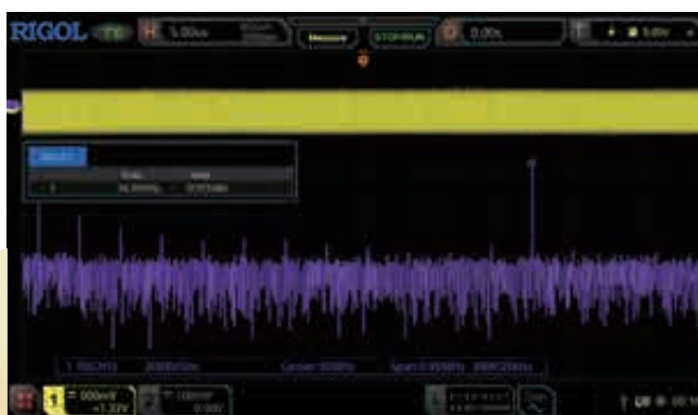
With the near-field probe, you can easily observe the spectrum peak in the frequency domain when the probe approaches to the radiation leakage point.
