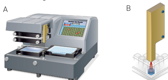
Figure 2. (A) The Agilent BioTek Verify technology is built in above the manifold. The Verify probe (B) sends ultrasonic waves into a microplate to determine the fluid volumes in each well following dispense and aspirate cycles.
