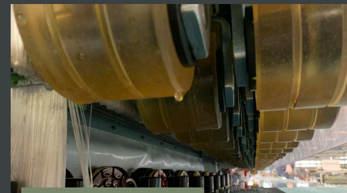
Doppie ruote pressore antimpronta (optional) Double non-marking pressor wheels (optional)
