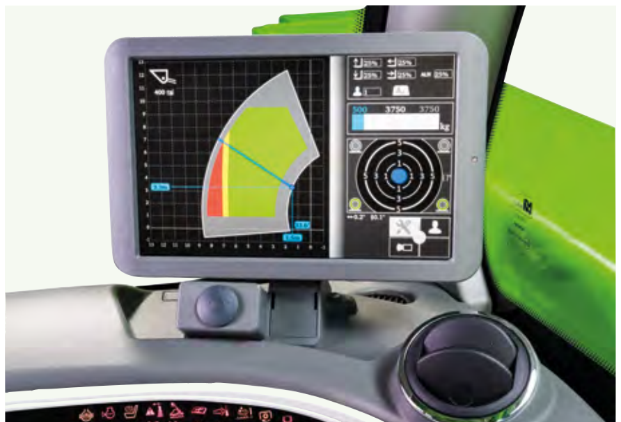
Merlo ASCS (Adaptive Stability Control System) rated capacity limiter
