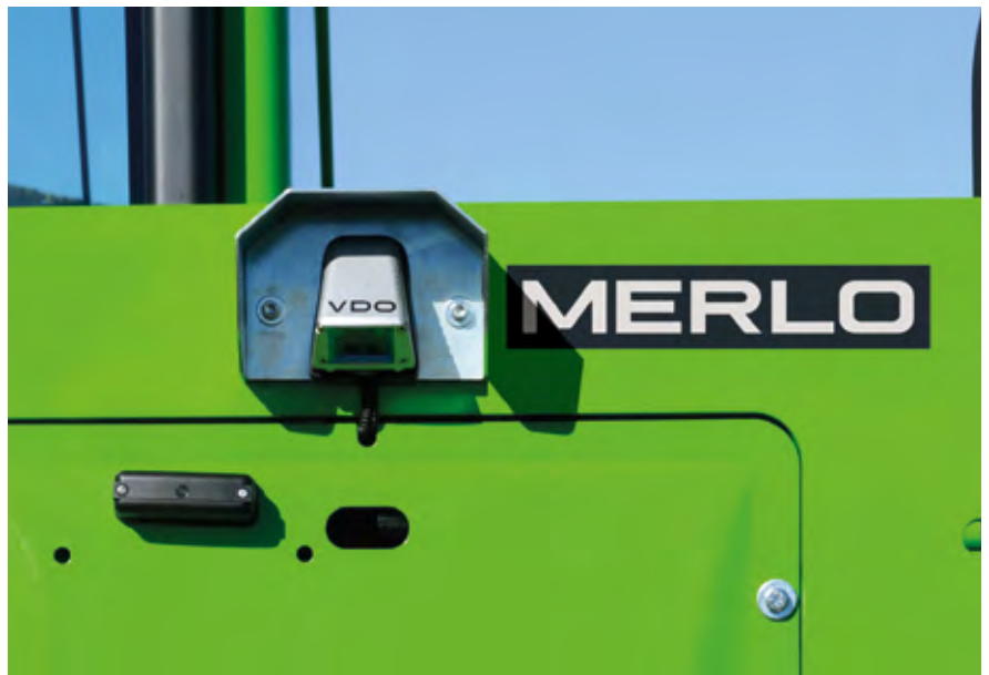
Rear camera starts automatically when engaging the reverse shuttle.
