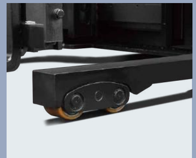
The structure of rotary load wheel offers the truck better passing ability
