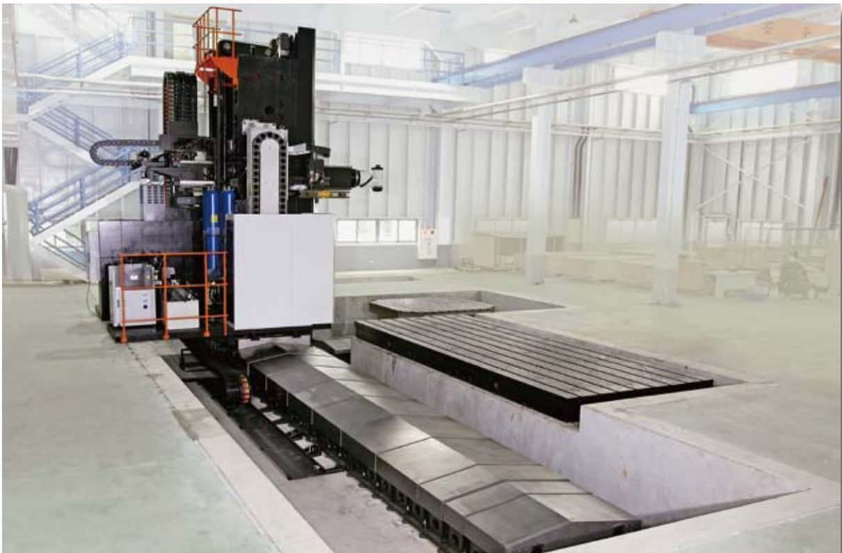
4. operator and serviceman walking into machine directly from the back side of machine with easy access
