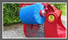
Large apron, set at an optimal angle, allowing control of material during screening
