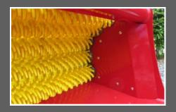
Massive screening area, with replaceable inner panels for machine longevity and shaft end discs for low running costs
