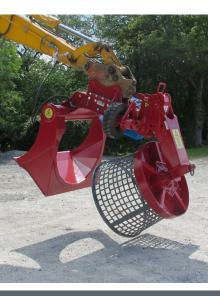
Interchangeable drums, from 10mm to 100mm, with cleaning brush fitted as standard.
