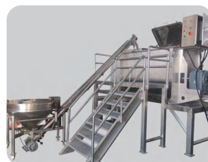
Different loading system: manual with platform and ladders, automatic with screw conveyor
