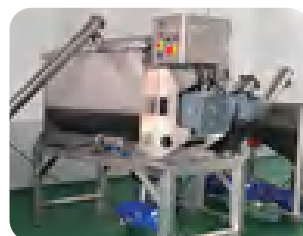
Different loading system: manual with platform and ladders, automatic with screw conveyor
