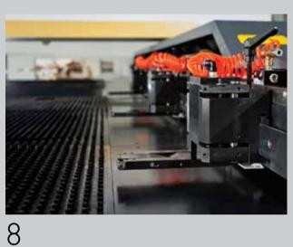
**CLAMPING** Movable pneumatic clamping.
