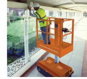
**Drivable at height** Interlocked rear gates as standard Superior platform height 3350mm TTTT No chains or pulleys in mast **Extended battery life** with maintenance free AGM batteries up to 30km's on one charge THE REPORT OF
