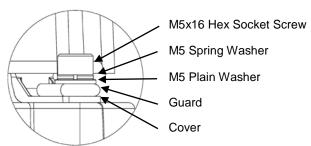
Fig. 13 Cover and Guard Fixtures
