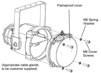
Fig. 2 Accessing the Explosion proof Enclosure.
