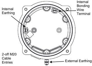
Fig. 3 Internal View of Cover
