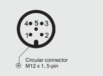
Connect the cable shield to the force transducer housing. In the case of accessory cables, the cable shield must be connected with the knurled nut and thus connected to the housing of the force transducer. When extending, only shielded and low capacitance cables should be used. The permitted maximum and minimum lengths of the cable are specified in ISO 11898-2. A high-quality connection of the shielding must also be ensured.
