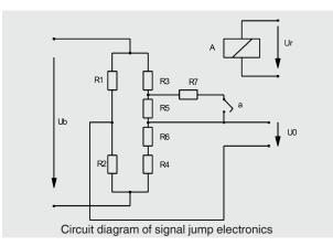
These force transducers are working with four variable resistors (R1 ... R4) connected to a Wheatstone Bridge. Caused by deformation of the body the respective opposite resistors are lengthened or compressed in the same way. This results in an unbalanced bridge and a diagonal voltage U0.
