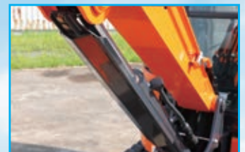
Boom cylinder guard The cylinder guard has a strong inverted V-shaped structure.
