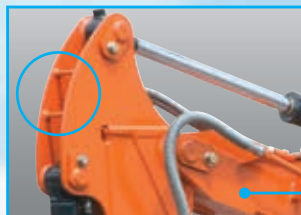
Hydraulic hose guard The bucket hose is covered with a guard, which prevents entanglement and interference.
