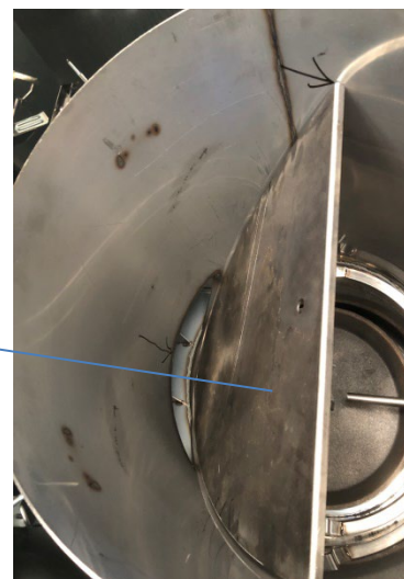
Fig. 3. Combustion chamber structure, profile left; Top view right, shows deflector position
