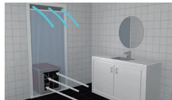
Negative room pressure is an isolation technique to prevent cross-contamination from room to room. It is generated and maintained by the air cleaner removing more air from the room than air is allowed into the room through the gap above the door.
