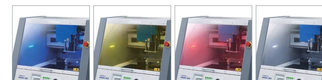
Colour-coded LED status lights
