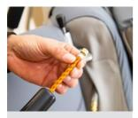
The backrest wings and seat arms should be rotated into the down position to best gain access to the valves. First remove the valve cap.
