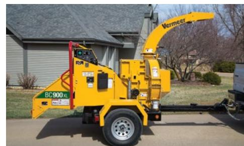
**EASE OF SERVICE.** This machine offers direct access to all parts of the chipper for routine maintenance without having to remove any shields. A dripless oil filter and five grease points are provided to reduce work effort and speed up service time.
