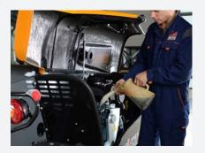
The engine compartment of the TENDO models are very accessible for daily checks of the oil, coolant and air filter.
