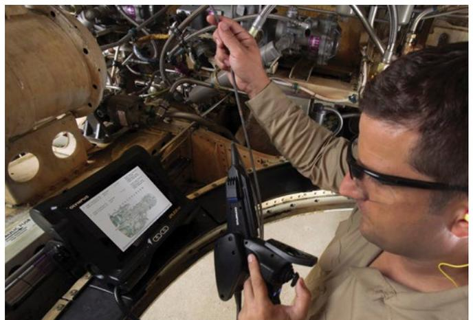
The IPLEX RX monitor displaying a manual PDF during inspection
