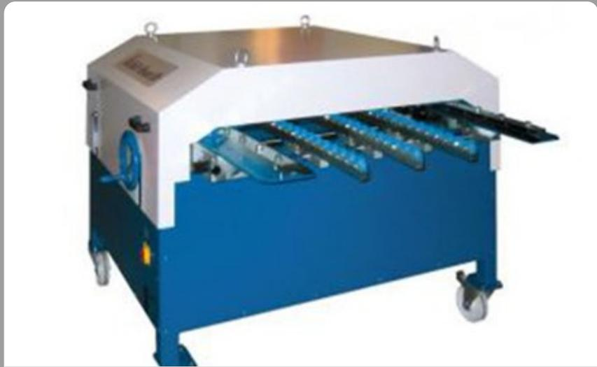
Angle Cutting Unit KONI2000 with decoiler AH1250A1
