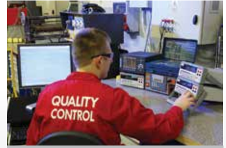
Final test of actual duty cycle, electrical safety, EMC
