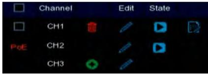
**PoE:** This represents the IP camera is connected to the PoE port of the eIVP model.
