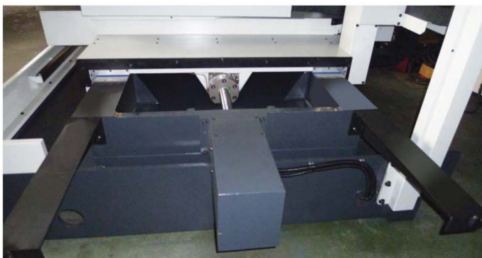
X/Z Axis Square Way Design / Z Axis Ball Screw Mounted at Central Slide
