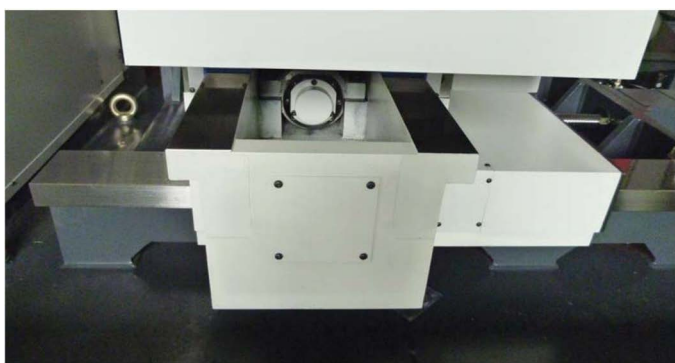
X/Z Axis Square Way Design / Z Axis Ball Screw Mounted at Central Slide
