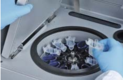
Removing rotor adapters
