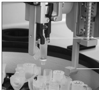
Fully automated spin-column processing
