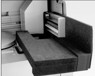
Foam protector inserted between the centrifuge and the robotic arm
