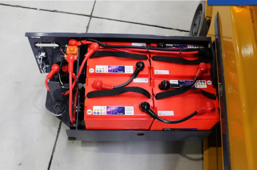
Maintenance-free batteries and easy motor access
