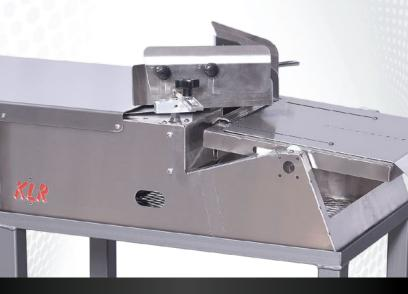
Overall dimensions: 8" H x 14.5" W x 45" L (adjustable stand for working height from 32" to 38") Product width: 10" maximum Electrical requirement: 120AC, 1PH, 1A Overall dimensions: 4" to 13", wicket bag only
