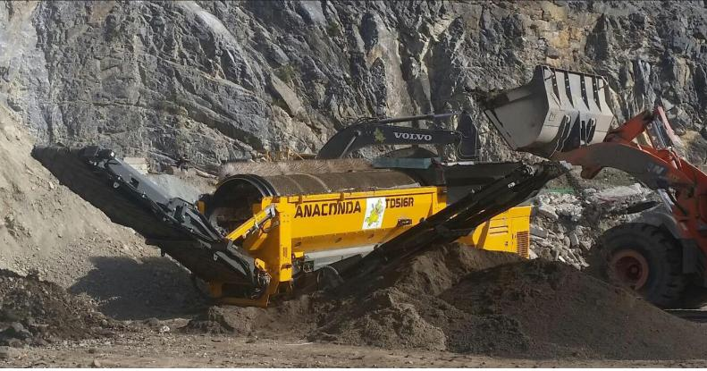
The Anaconda TD Range of Mobile Tracked Trommel Screens are Heavy Duty Cylindrical Screens that have been designed specifically for exceptional results in testing scenarios.
