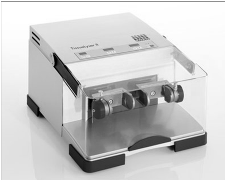
Figure 1. TissueLyser II (closed). The transparent hood is lowered, and the clamps at the front of the instrument are empty.
