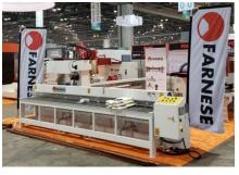
FARNESE AUSTRALIA recognizes the high demand from consumers for elegant stone features and the Stone Industry's need to make clean, quick and accurate mitres to meet this demand. The MITRE SAW simply and speedily cuts accurate mitres for a wide range of materials including engineered stone, granite, marble and porcelain of thickness ranging from 8 to 40mm.
