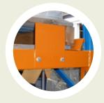
Pallet stops are fitted to ensure that pallets do not extend beyond the rear of the drive-in rack.
