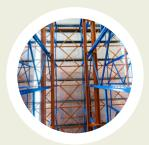
Cross Bracing are installed to the rear and top of the drive-in rack system for ultimate stability.
