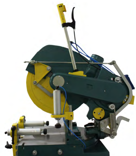
Figure 7. Saw Safety Guard & Locking System
