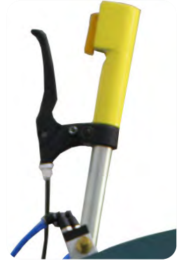
Figure 8. Saw Handle with "Dead Man" Trigger Switch
