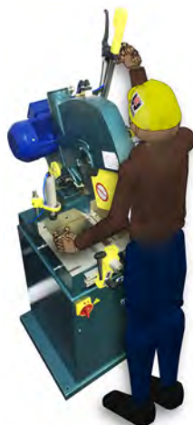
Figure 5. Correct Position for Operating Saw Unit
