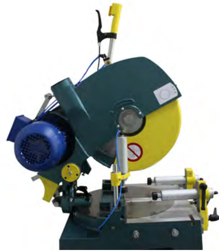
Figure 6. Main Function Motor Location (dark blue)
