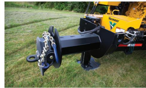
**JOB SITE MOBILITY.** The WC2300XL has a compact design and built-in skidder grab on the tongue, allowing it to be moved around on the jobsite by a skidder or excavator.
