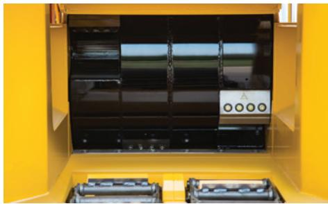
**OPTIMAL CUTTING PERFORMANCE.** Two knife options, with depths of cut of 3/8" (1 cm) or 5/8" (1.6 cm), allow the operator to select the knife that meets their end-product sizing needs.
