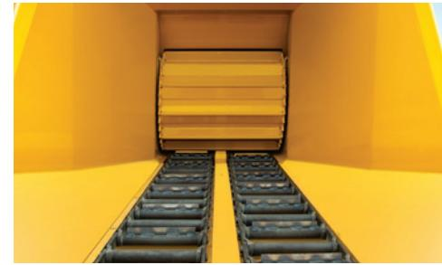
**INCREASE PRODUCTIVITY.** With technology such as SmartCrush to automatically increase down pressure when difficult material enters the cutting drum, and the variable-speed dual-infeed conveyor chains, operators can concentrate on loading the machine, not pushing the material through.
