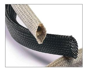
This high flame-retardant and halogen-free expandable braided sleeving is manufactured from modified polyester monofilament which is in compliance with UL94V-0 requirements.
