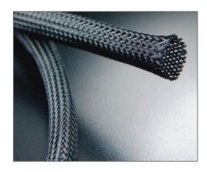
PPS expandable braided sleeving is made from polyphenylene sulfide (PPS) monofilament. It is used in high temperature environments and is known for its resistance to acids, solvents, fuels and abrasion. It also has high temperature stability, low moisture absorption, and excellent dimensional stability.
