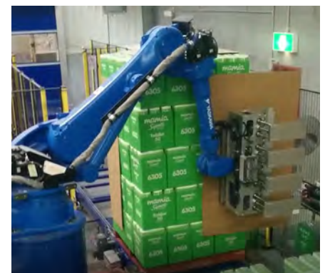
Automation of Corner Protectors
