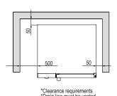
Heat Source: 500mm clearance from an external heat source is required in order to protect the oven control components and allow access to the service panel. For clearances under 500mm, it is mandatory for Stoddart heat shields to be fitted while still maintaining a minimum clearance of 300mm to provide access to the service compartment. Failure to adhere to minimum clearances may void the oven warranty or add service costs due to lack of access.
