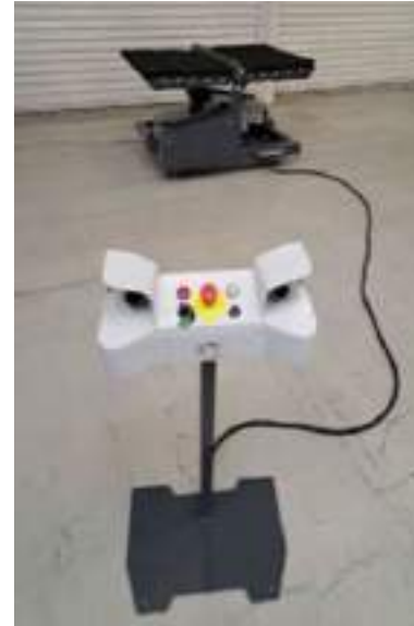
Two-hand pedestal control for Pneumatic EasyFlipper
