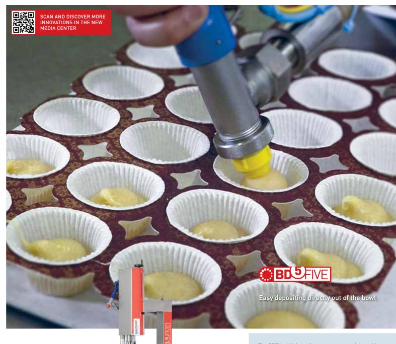
The BD5 is a high-performance pump and depositing machine that deposits your products with great accuracy. This BD Depositor is easy to handle and is easily movable on swivel casters.
