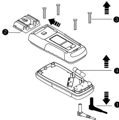
Fuse type : 11A/1000V – 20KA (10x38mm)
