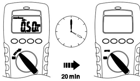
Wake-up the meter by dialing the switch or pressing any button.
