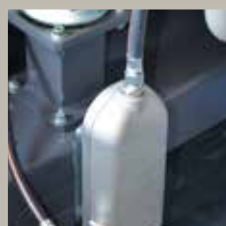
Engine heater warm up the engine to make starting easier
