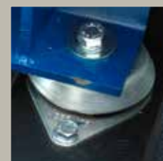
Mounting pads they allow to attenuate the vibrations emitted by the operation
