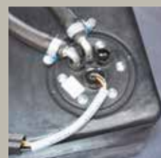
Automatic stop system due to lack of fuel with reserve signal
