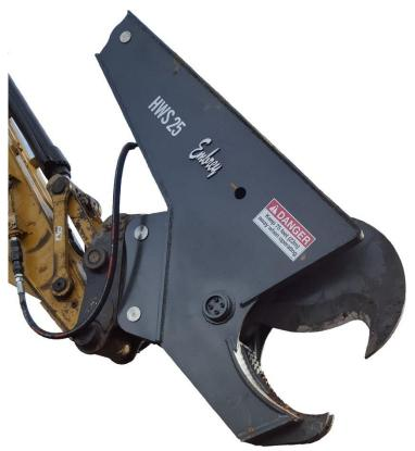
The *Embrey* Hydraulic Woodshears are designed for Land clearing, wood waste recycling and the downsizing of tree stumps, logs, sleepers etc. The new moving jaw is now milled from one piece of high tensile steel with a sharper cutting angle than previous models.
