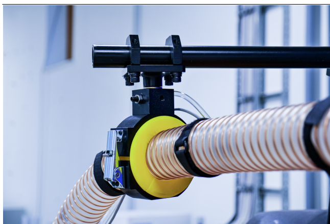
Assembly example of hose routing for vacuum grippers on industrial robots
