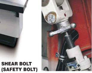
Should the knife strike a hard material, shear bolts are broken to avoid serious damage to the machine.
