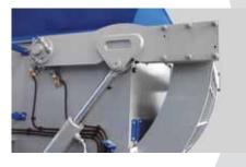
The ZSS series shredders benefit from sturdy ram construction incorporating heavy duty guide bearings and universal couplings for reliable operation.
