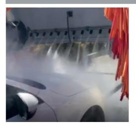
Oscillating sides high pressure system + top scanning high pressure system.
