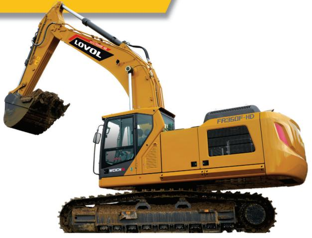
The LOVOL 37 tonne ALFA series excavator features a tier 3 Deutz Weichai engine and a Linde hydraulic system with pilot oil operated joysticks for precise control. Heavy duty construction and renowned reliable componentry saves you downtime and costly repairs.
